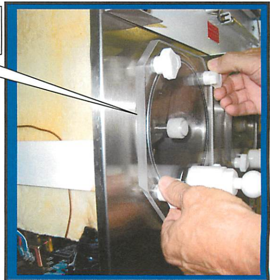
Installing faceplate C6521 onto front of Machine.
