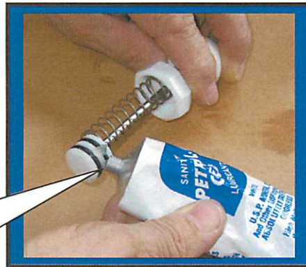
Installing o-rings onto plunger F 0491
